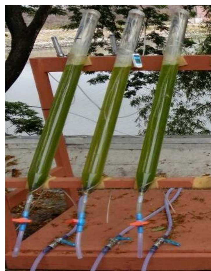
Figure 2 – Schematic of the glass-made 3-liter cylindrical type photo-bioreactors and used in this study.
